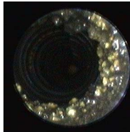
EG/DI Water with a Cation Exchange Bed (ion exchange particles)
