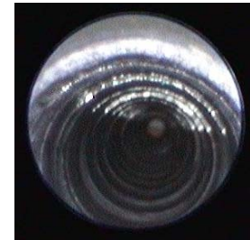
Dynalene FC with nanoparticles (no deposits or corrosion debris)
